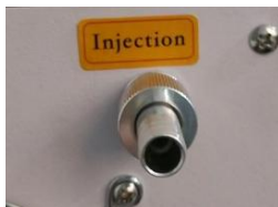
Fill water position
