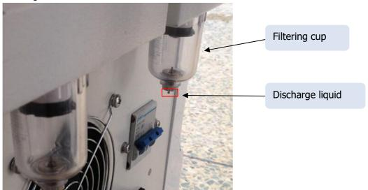
When the filtering cup full, please discharge liquid in cup through extruding this button.
