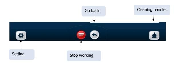
**Cleaning handles:** touch this icon for cleaning handles, in avoid the oil blocking the vacuum pump. cleaning time is 30 seconds.
