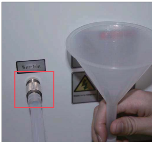
7. Connected the filling funnel and tighten it, add water until the Water Overflow come out of water, then it's completed
