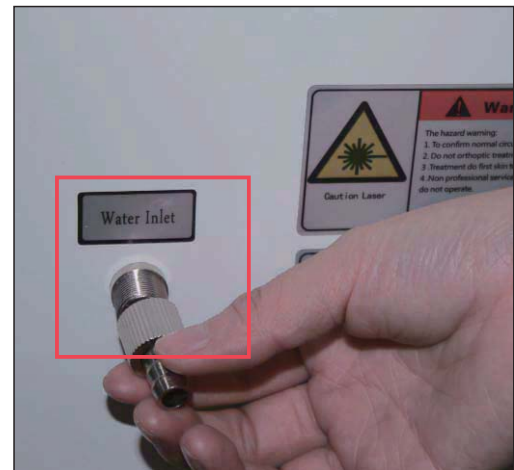
8 . After add water , pull out the filling funnel ,then cover the nut
