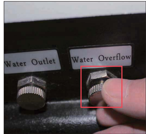
6 . Screw off water overflow nut
