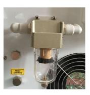
If oil is over 1/3 level of the filter, take off the filter, discard the oil, then put back the filter
