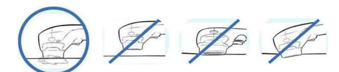
The cartridges must be horizontal.
