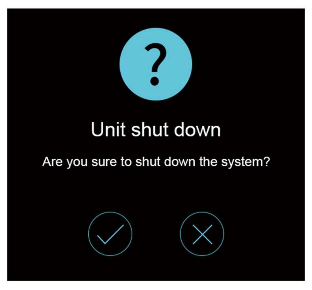
After touching "OK", a small pop-up window as below will pop up on the interface(it prompts "After each treatment, please wait 5-8 minutes before turning off the master switch! To ensure that the internal system circulation cooling!) Please wait 8 minutes before touching the "confirm" button.
